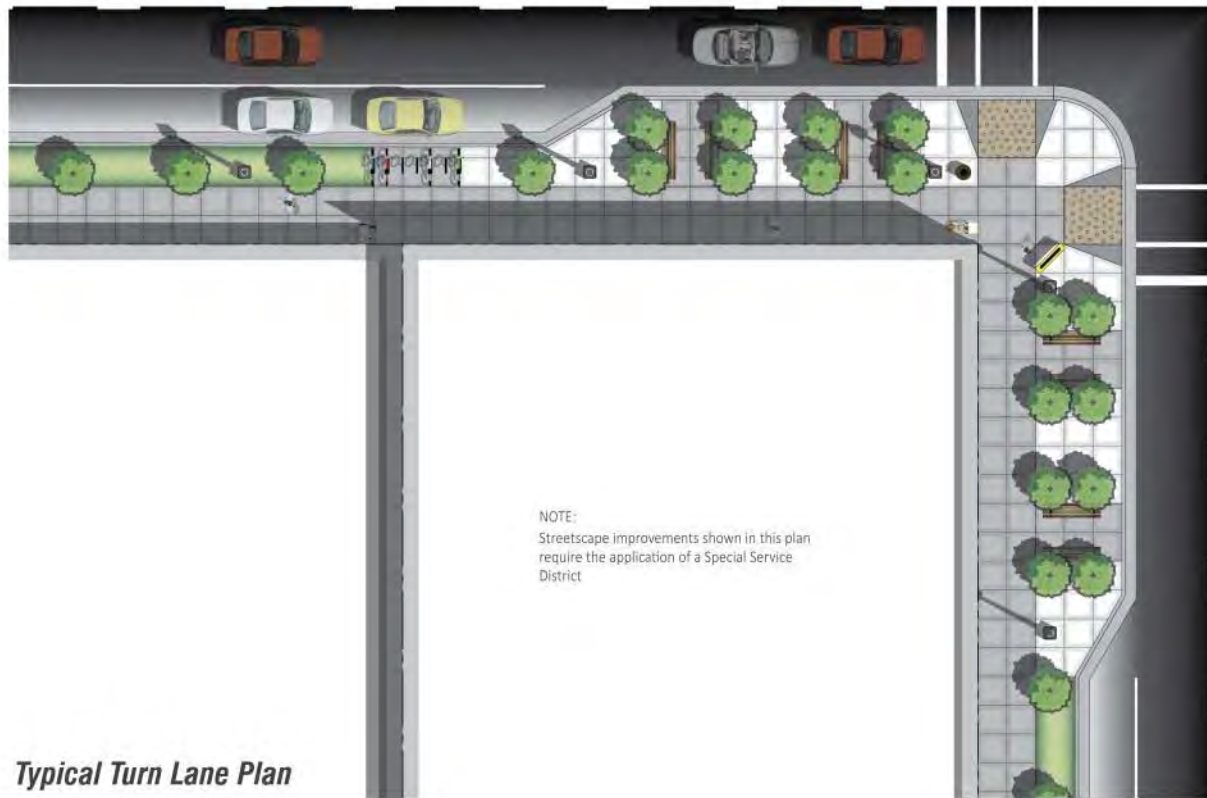
Figure 5.2 - Recommended Intersection Streetscape Design – with Bump Outs
