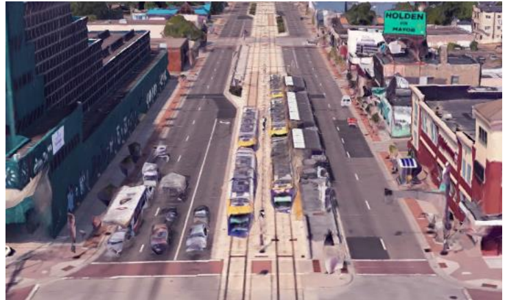
University Ave and Snelling, showing a 2-lane street design in each direction. Example for the suggested changes to Highway 55.
